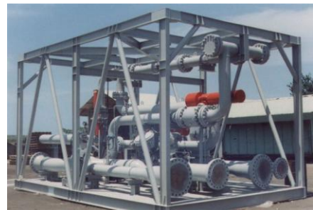
Developed Subsea Pressure Boosting System Increasing Production by 30%
