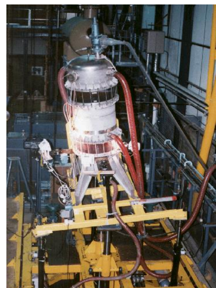
Vertical OW/G Separator being Tested on BHR 5 Degree of Freedom Rig
