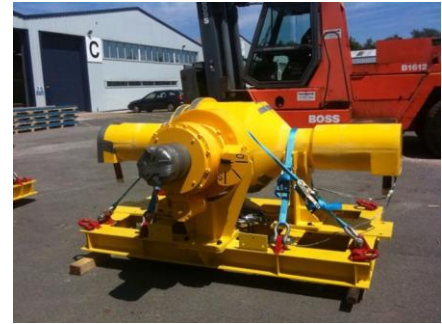
Subsea Valve Being Made Ready for Thermal Cooldown Qualification Test
