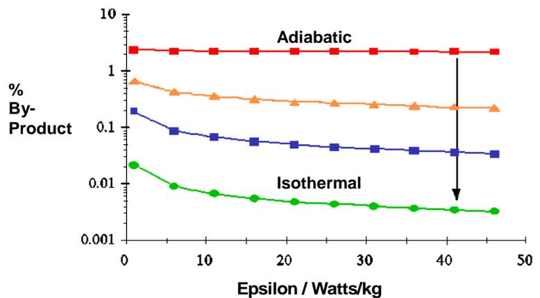
By-product formation decreases as mixing intensity and rate of heat transfer increase. As more reaction heat is removed, mixing benefits become even more pronounced. Trends can be predicted for industrial reactions by our experimentally validated model.
