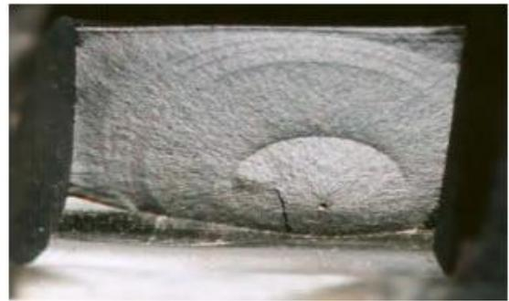
RGD Fatigue in Elastomer
